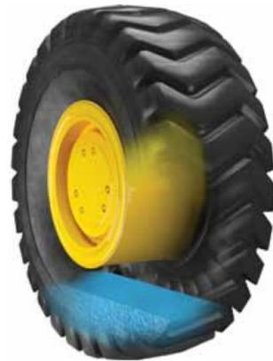
TLC Tire and Rim Protection conditions the wheel and maintains cooler tire operating temperatures. The liquid is added to the tire air chamber and coats the inside of the rims to provide rust protection. TLC's rust inhibiting formula, superior coating properties, and continual vapor dispersion extends the life of tires and rims. Plus, TLC is non-toxic, non-flammable, and non-hazardous.
