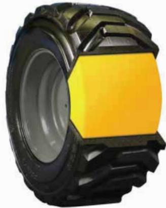
TyrFil® is a patented polyurethane material that is pumped into OTR mining vehicle tires, replacing all the air. It cures into a flexible, durable filling that acts as a shock absorber and completely eliminates flat tires. Compared to other flatproofing products such as solid tires, cores and liners, TyrFil is the most cost-effective solution and provides the best overall performance.
