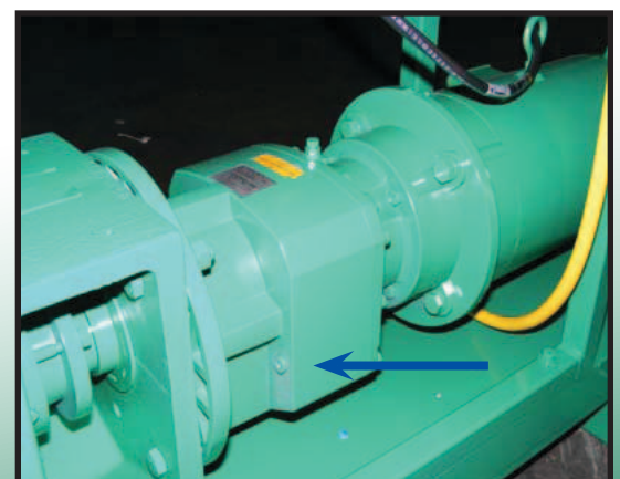
Progressive Cavity Mixer Motor Location: Directly under the control panel chassis
