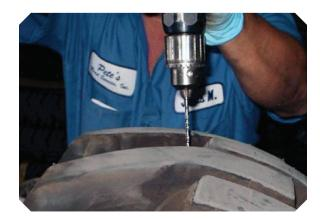
**Step 9.** When foam fill starts flowing out of weep hole continuously, plug weep hole with screw or nail.
