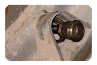
**Step 3.** Insert valve core into fill gun plunger shaft making sure it is completely seated in the holder. Make sure plunger is completely pulled back to the rear of the fill gun.
