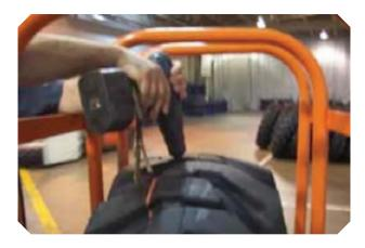
**Step 6:** Fill tire until fill starts to come out of weep hole and all air is out of tire and fill runs continuously.
