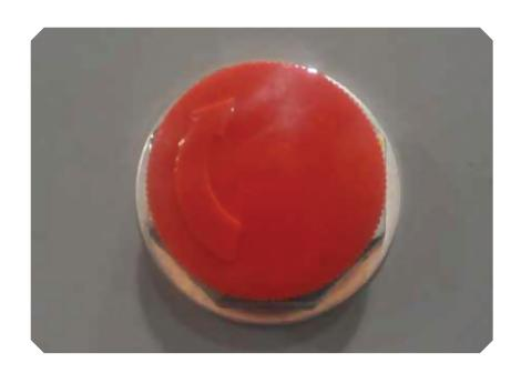
STOPS ALL OPERATIONS OF THE MACHINE AND PLACES THE INVERTERS INTO EMERGENCY STOP MODE
