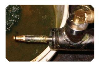
**Step 4.** Attach gun body to fill gun adapter assembly on valve stem.
