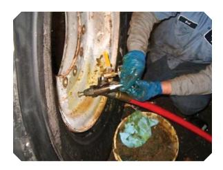
**Step 14.** Remove fill gun body from fill gun adapter assembly.
