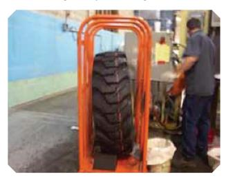
**Step 2:** Drill a hole in the side of the tire on the opposite side of the tire as the stem. Stem should be at the six o'clock position and the hole position should be as shown. *Note:* always fill tires from the bottom up.
