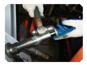
**Step 13:** Loosen coupling and unscrew needle from plug.
