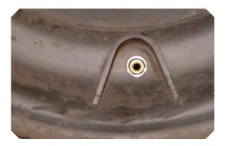
**Step 2.** Thread the fill gun adapter on to the valve stem until completely seated (do not over tighten, just snug).
