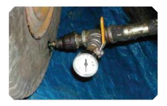
**Step 9:** Fill tire to within 10 psi of recommended pressure.
