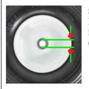
STEP #4 Measure the inside diameter (I.D.) of the bore
